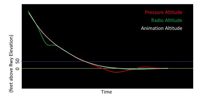
However, this assumes that the aircraft *is above the runway elevation at 50 feet*. If for example, the aircraft lands short and there is a valley before the runway threshold, this method will not work as the valley will result in an increase in height that will show the aircraft rising when it did not as shown in the yellow line in the figure.
