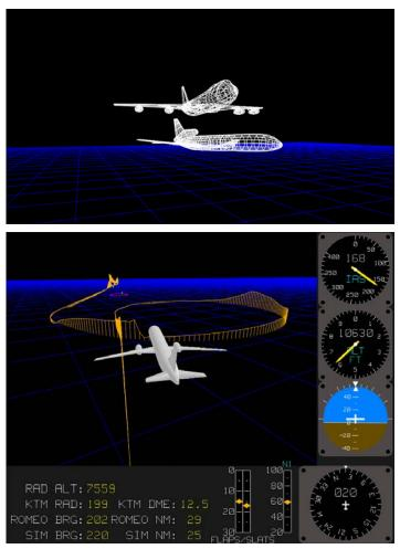
we did at the time (around 1990) had a very simple terrain profile by subtracting pressure altitude from radio altitude – which is the orange line you see under the flight path. The instrumentation was very simple compared to the primary flight displays and other avionics displays in today's cockpits.
